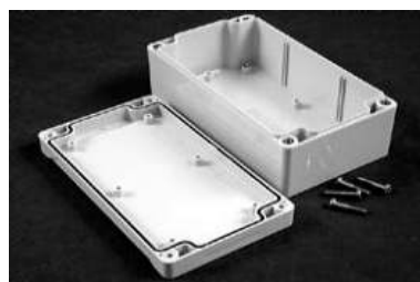
26-1555 Series Recessed lid for membrane keypad & PCB spacers moulded into lid - designed for #6 self-tapping screws.
