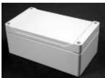
26-1555 Series Recessed lid for membrane keypad & PCB spacers moulded into lid - designed for #6 self-tapping screws.
