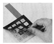
3. Remove the separator paper from the top of the switch then carefully place the overlay onto the adhesive on the switch.
