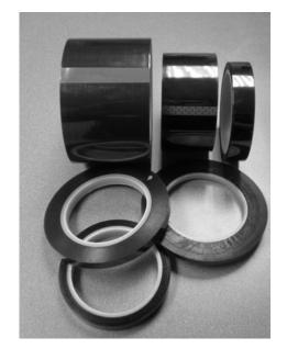
**Kapton Tape** is 1 mil thick and has a 1.5 mil silicone adhesive and will withstand temperatures of up to 260°C.
